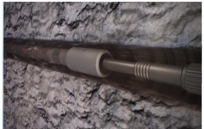
The AVD can be run in the BHA below the Jars. It is as strong as the drillpipe and no surface intervention is required to activate i.e. no balls or darts. If the BHA becomes stuck, the Operator can achieve a disconnect in a matter of hours depending on how the AVD has been programmed.
