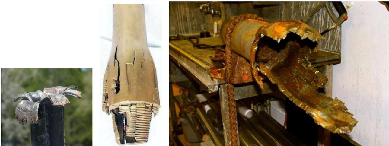
Figure 1 – examples of severed Drillpipe.
