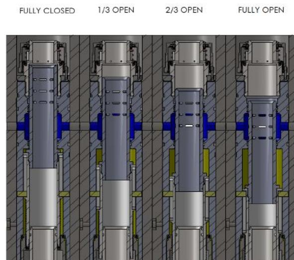
Figure 6 – Circulating Valve positions
