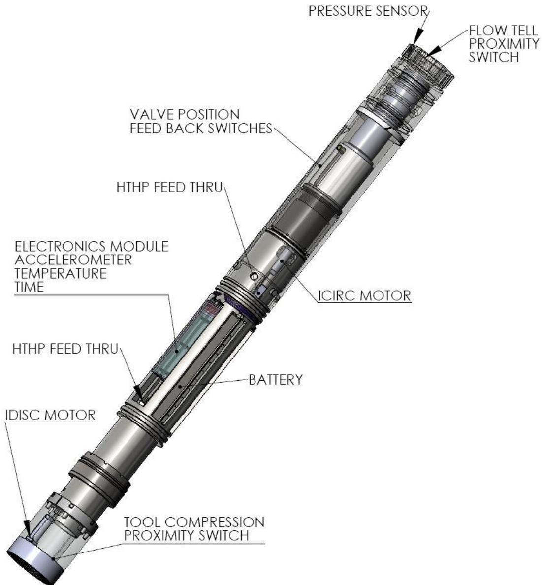
Figure 2 – Electronic Service Module
