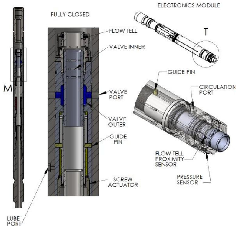
Figure 5 – Circulating Valve layout
