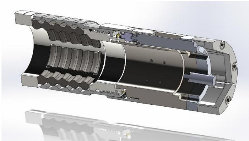
Figure 8 – Section through Clutch
