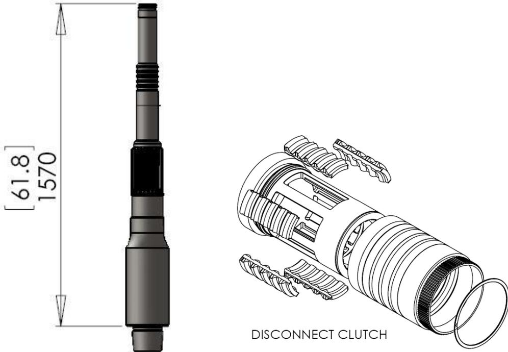
Figure 7 – Clutch Mechanism
