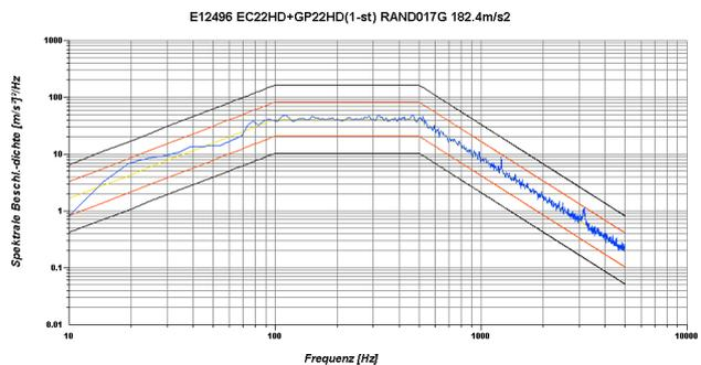
Figure 9 – Graphs of Motor reliability testing, 2000hrs operating at 180 degC at up to 17G vibration levels
