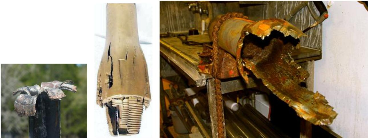
Figure 1 – examples of severed Drillpipe.
